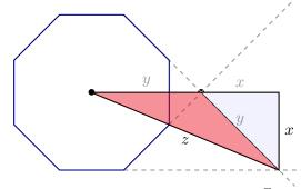
By the Pythagorean Theorem,  $z^2 = x^2 + (1+\sqrt{2})^2 x^2 = (4+2\sqrt{2})x^2$ . Earlier we saw  $z = \frac{x}{\sqrt{1-x^2}}$ , so we can equate two formulas for  $z^2$ .
